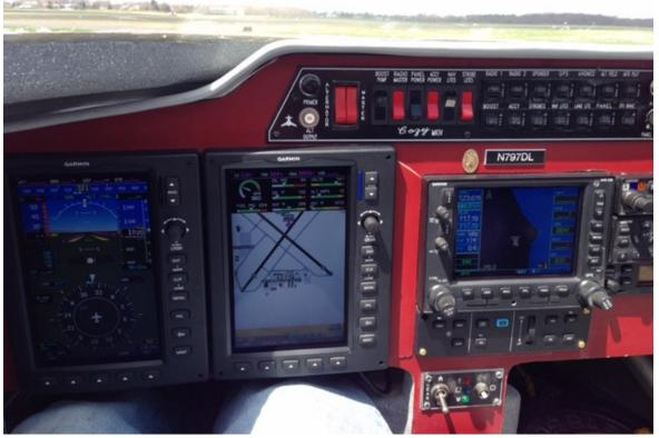
Garmin recently came out with a software release that provides a 'new feature' previously only available on the G1000's for Cirrus. The feature is called ESP (Electronic Stability and Protection). It's similar to what the Airbus and Boeing EFIS's have to keep the aircraft within predefined parameters.... so what's that mean. It means the software will stop the pilot from getting the plane into an 'unsafe' attitude or airspeed.
